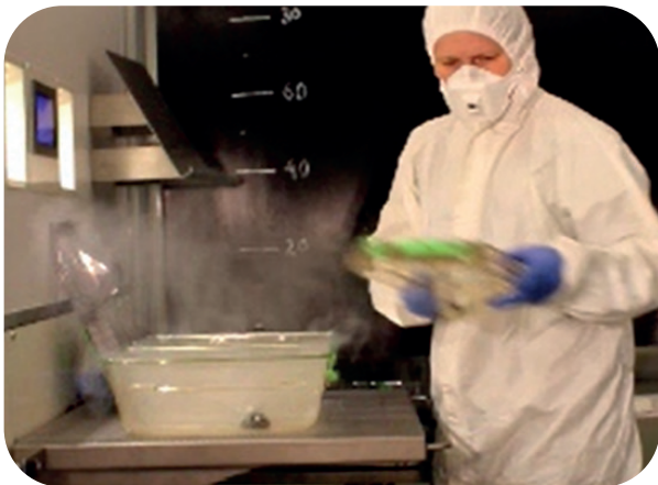
Environment: The downflow and inflow ensure that no allergens nor pathogens leave the cabin (this image was taken during a smoke test).
